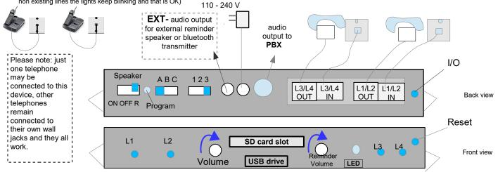
Turn the speaker ON to confirm audio is playing and adjust the volume to mid level (if device is not activated yet or it has stopped LED goes RED and there would be no audio playback - if so refer to Quick Start & activation sheet or P7)
